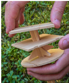
Production via CNC Cutting of the 1:10 scale model and demonstration of the interlocking of the various pieces
